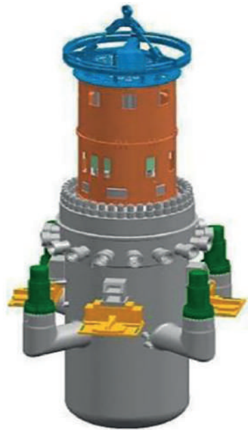
Figure 3 ACP-100 Reactor Vessel (Deng et al., 2020)
