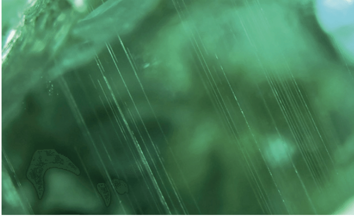
Şekil 17. Musakashi zümrüdünde, kristalin prizma yüzeylerine paralel büyüme tüpleri https://www.researchgate.net/figure/Growth-tubes-parallel-to-the-prism-faces-of-the-crystal-are-visible-in-this-Musakashi_fig3_264542547
