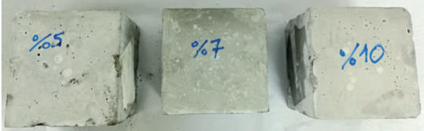
Fig. 5 Blocks produced by adding 5%, 7%, and 10% cement to the waste powder
