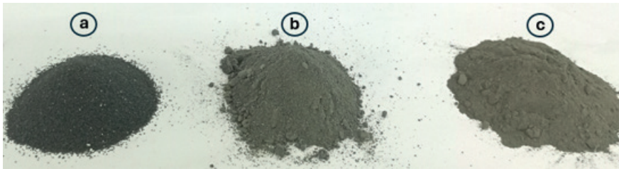
Fig. 4 a) Corundum abrasive, b) BAR test-derived waste powder, c) its ground form
