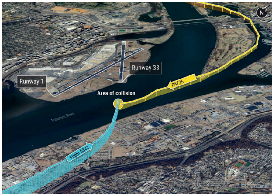
Figure 7. Reconstructed flight trajectories of PSA Airlines Flight 5342 and U.S. Army Priority Air Transport Flight 25 (PAT25) during the final approach phase near Ronald Reagan Washington National Airport (DCA), illustrating the convergence of commercial and military flight paths immediately prior to the mid-air collision. (Adapted from National Transportation Safety Board [NTSB], 2026).
