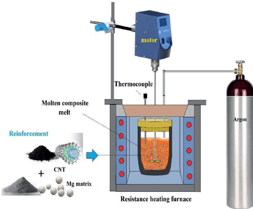
*Fig. 6. Liquid Metallurgy route for manufacturing NRMMCs [1]*
