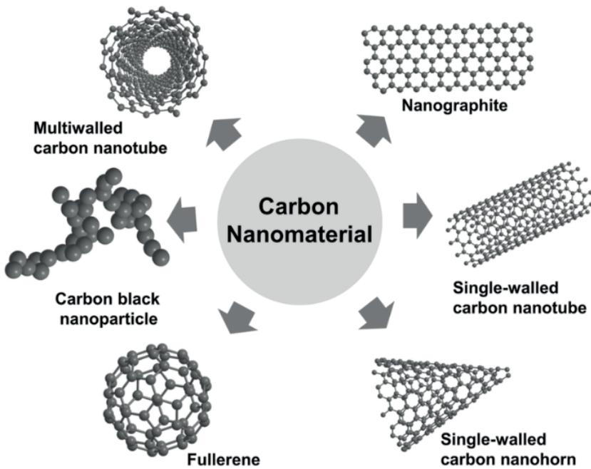
*Fig. 3. Carbon nano materials used in NMMRCs [3]*
