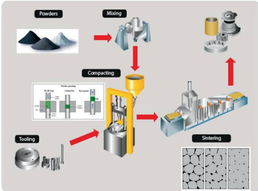
*Fig. 5. Powder Metallurgy route for manufacturing NRMMCs [23, 27]*
