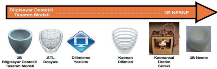
Figure 1. Production process of 3D printers
